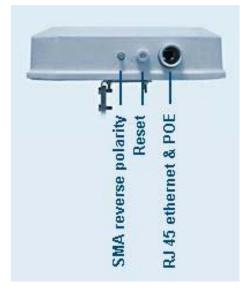
by telnet. It uses a TCP/IP protocol base. The radio components work in the 5,2 to 5,8 GHz band, and are compatible with the IEEE 802.11a standard.
